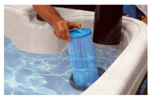
Unscrew the cartridge and remove it.
