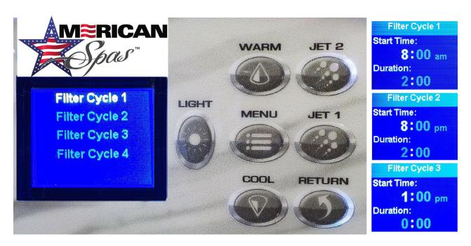
Filter Cycles 1, 2, 3 and 4 can all be adjusted in 15 minute increments. Use the MENU button to move from field to field, use the UP and DOWN arrows to make adjustments and then press RETURN once you're satisfied with your selections for all Cycles. Please note that the system will not allow you to set overlapping or contradictory Cycles.
